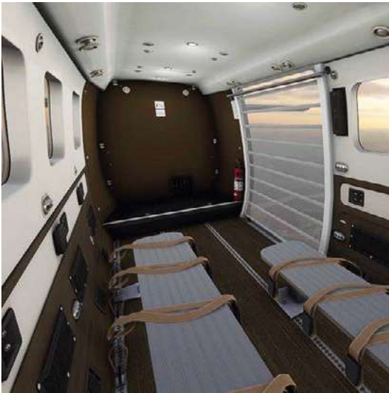
These interior photos show Daher Engineering Services' modifications to a Kodiak 100. The new headliner access panel for the skydiver door closure mechanism is shown above, and the new aluminum side-fuselage skydiver door is highlighted at right.
