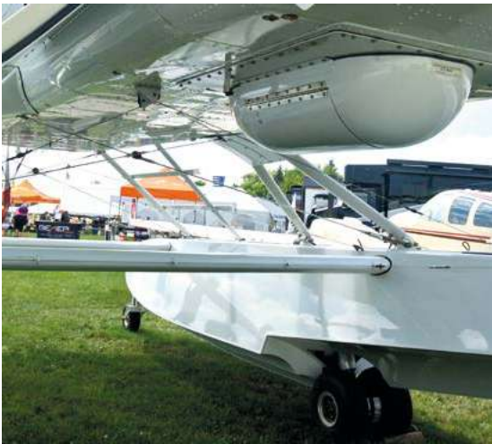
The Kodiak 100’s underfuselage fairing protects the sensors that can be installed in the aircraft for its survey missions. Also visible in this photo is one of the Aerocet 6650 amphibious floats with its landing gear extended
