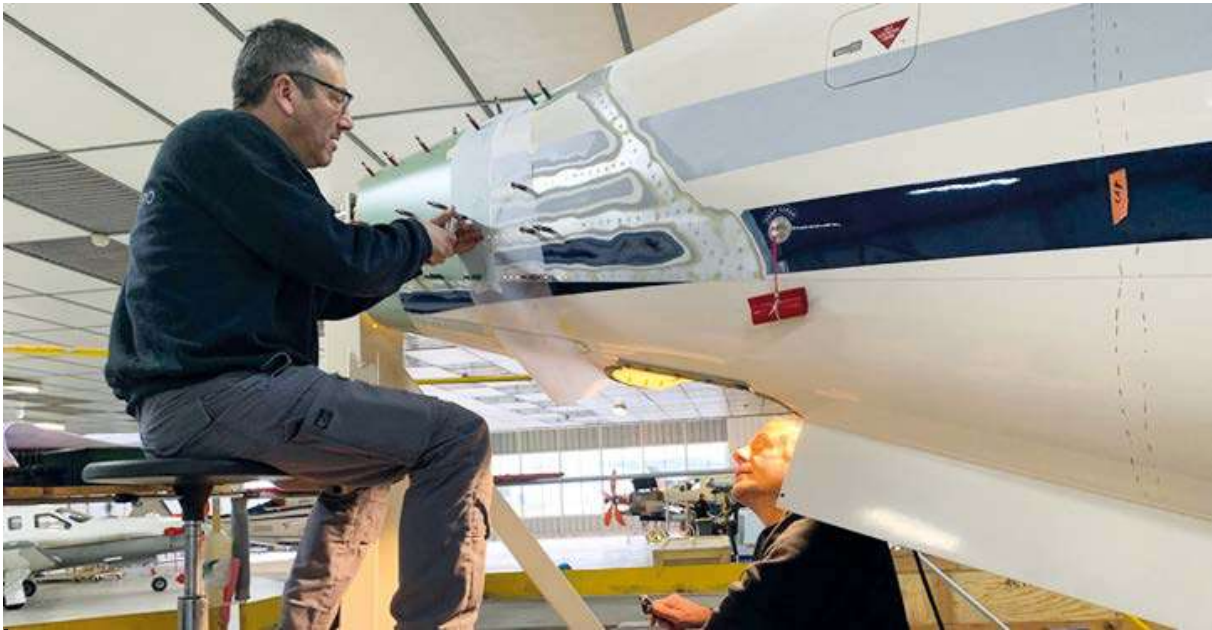
Members of the Daher Engineering Services team perform a tailcone repair on a TBM 850 that was involved in a ground handling incident. The TBM's fuselage is installed on a jig adjusted to the same tolerances as on the TBM final assembly line, ensuring high accuracy for the repair work.
