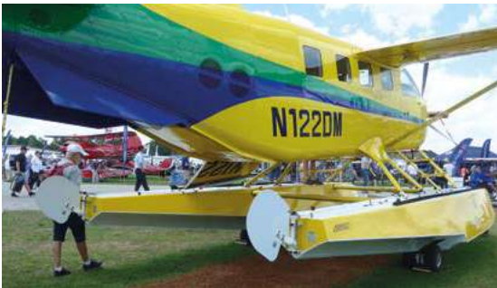
Features of Aerocet’s Kodiak 100 floats include a double-fluted design that provides superior strength-to-weight ratings, as well as sharp edges for reduced drag and increased hydrodynamics.
