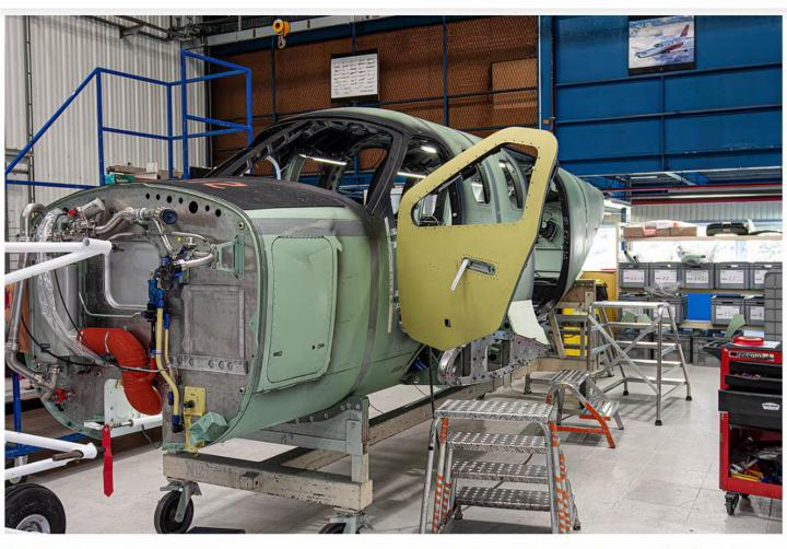
The fuselage of a TBM 900 series prior to gaining its wings and Pratt & Whitney PT6. [Credit: Stephen Yeates]
