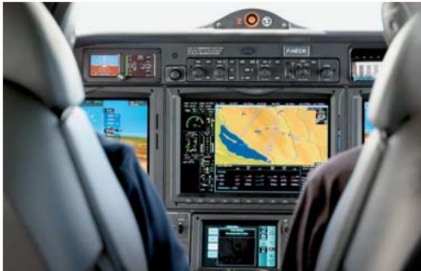
The Garmin 3000 cockpit of the TBM 940 with the orange "Homesafe" button in the middle.
