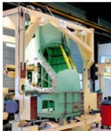
The cockpit sections of the TBM are built in a vertical position.
