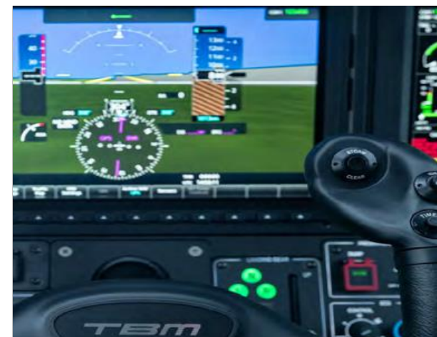
Flight Envelope Monitoring Aural Alerts for Stall and so on Stick-Shaker to warn an imminent Stall
