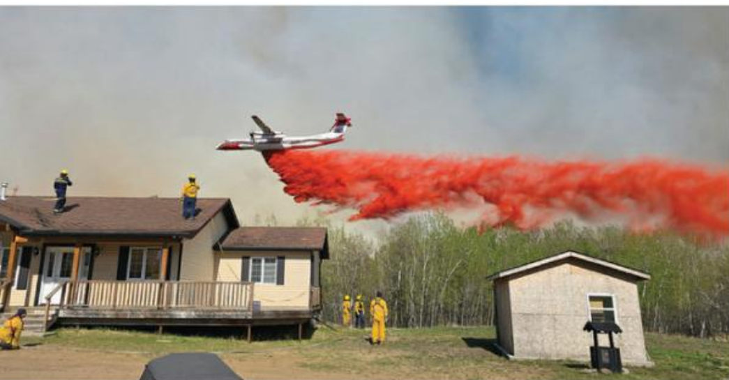
The Dash 8-400 air tanker is a versatile aircraft designed for aerial firefighting and other emergency response missions. The air-tanker-only variant can tackle wildfires with a 10,000-liter (2640-gal) retardant payload, while the multirole version is designed to be reconfigured for different roles, including air tanker, cargo, passenger, and medevac. Photo by firefighter J Van Der Leek.
