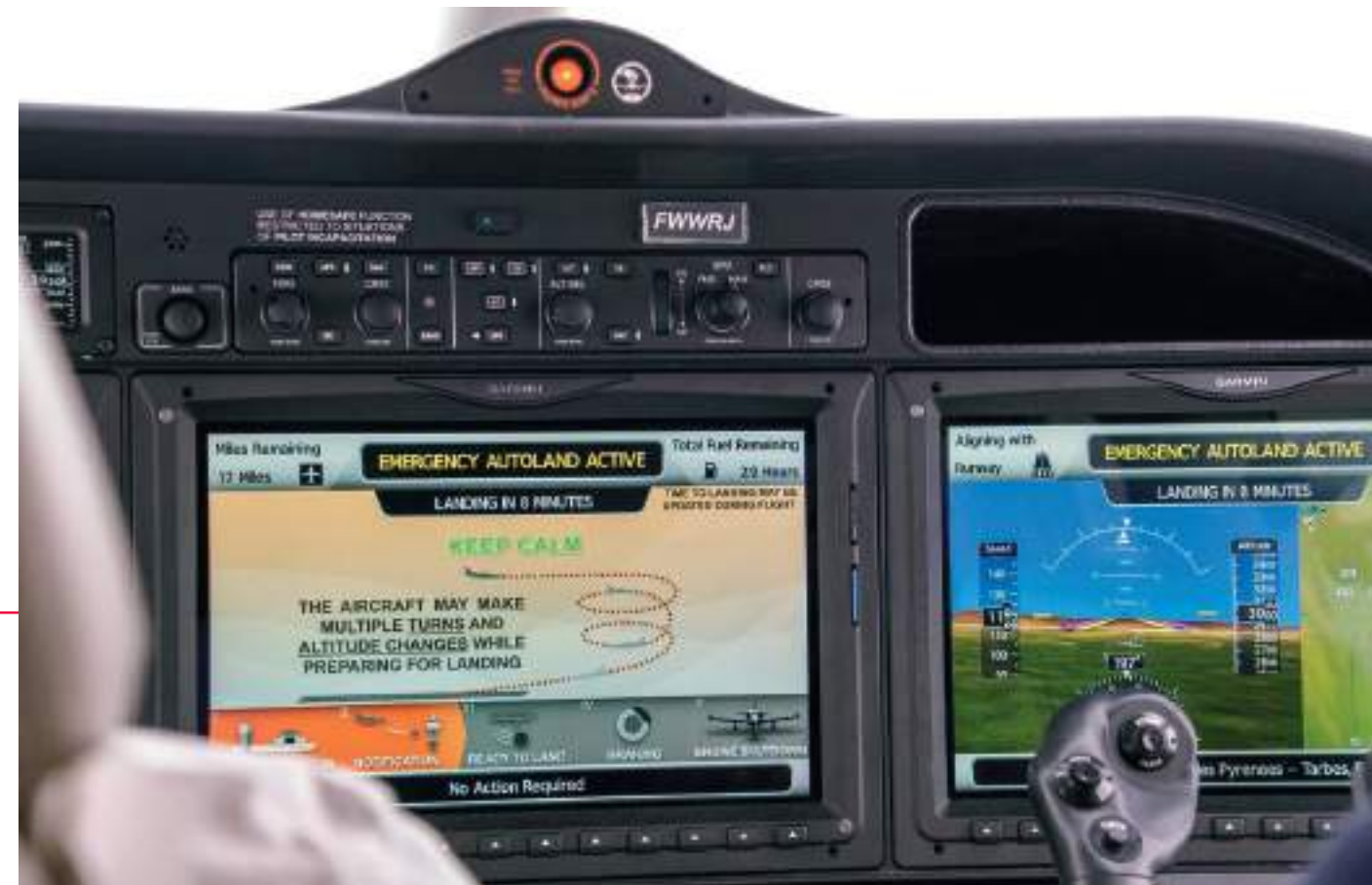
The video briefing that appears on the TBM 940 cockpit's multifunction display informs – and reassures – passengers after the HomeSafe™ emergency autoland system is engaged.
